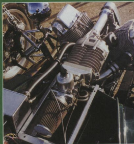
The rear aluminium cover lifts off to reveal the 1 3/4" SU carburettor and air filter lying neatly on the tunnel top.
