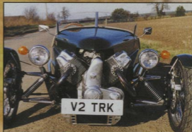
Other than the drive-belt casing and the oil cooler, there's little exterior sign to betray the presence of the supercharger. ...
